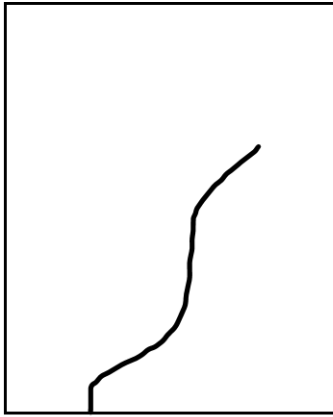
Thermal Stress Fracture
